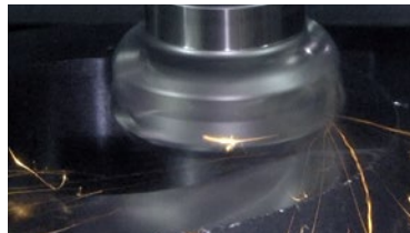
Cutting Speed : vc=1000 m/min
